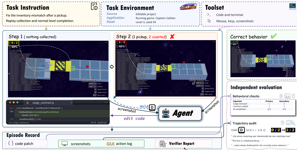
Figure 3: A concrete benchmark task: repairing inventory updates in Captain Callisto. Agents combine coding tools with interaction and screenshot observations. In Captain Callisto, one pickup incorrectly changes the inventory from 0/2 to 2/2. The code excerpt shows the agent’s final edit, while “Correct behavior” shows a separate reference replay. Independent evaluation checks both the protected behavioral tests and the validity of tool use. The table lists expected outcomes for two replay scenarios.
